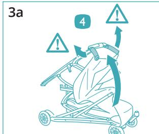
Pull handlebar toward you and adjust into place as shown (Figures 3a and 3b).
