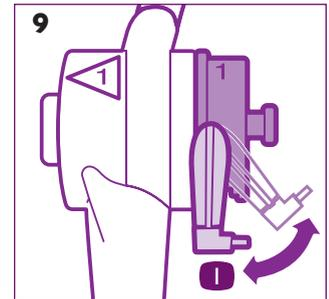
To reattach seat adapters, open stroller frame, lift up on grey tab to expose slots, align slots with frame, slide adapters in and push down on grey tabs (Figures 9-9a).
