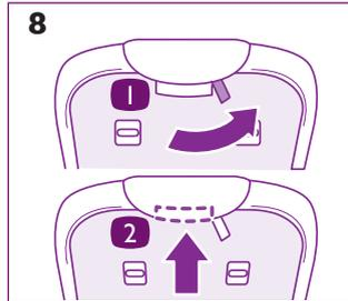
Rotate release tab outward, then squeeze recline button in all the way (Figure 8). While squeezing recline button in and while tab is rotated out, lift seat off frame (Figure 8a).
