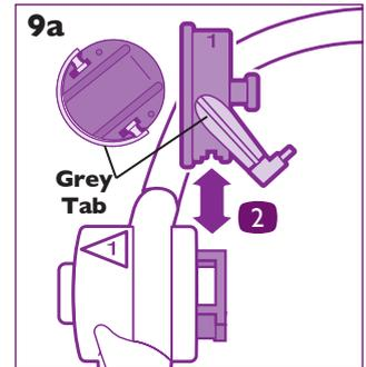
**NOTES:** Seat adapter labeled 1 fits into frame hub labeled 1. Seat adapter labeled 2 fits into frame hub labeled 2. Numbered adapters and frame hubs match up only when frame is in the open and in-use position.
